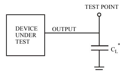
\* Includes all probe and jig capacitance
