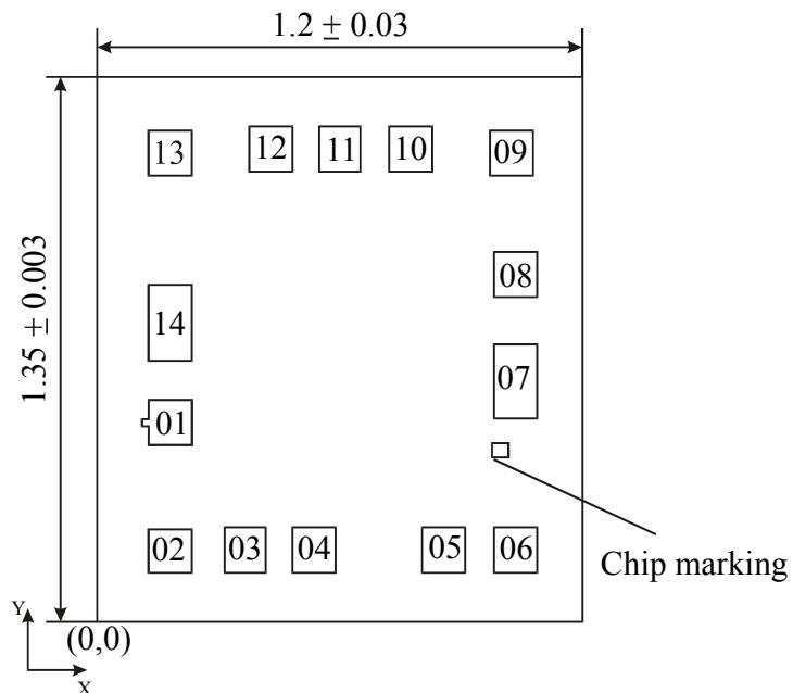
**Chip marking :15-32****Location of marking (mm):** left lower corner  $x = 0.978$ ,  $y = 0.411$ ; right lower corner  $x = 1.02$ ,  $y = 0.447$ **Chip thickness:**  $0.46 \pm 0.02$  mm
