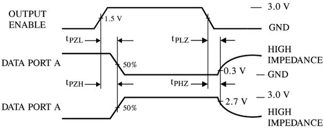
Figure 5. Switching Waveforms
