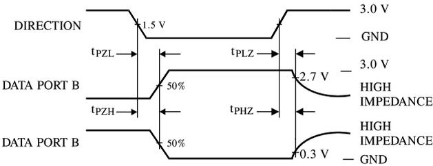
Figure 6. Switching Waveforms
