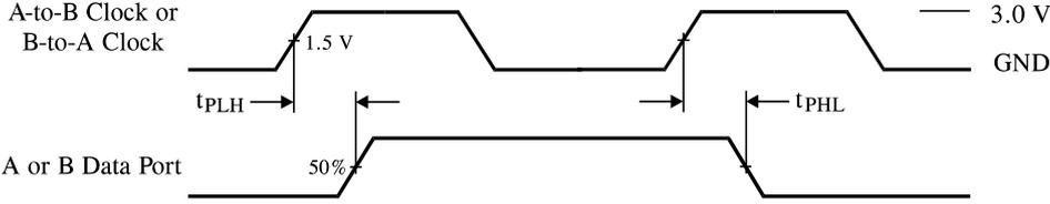
Figure 1. Switching Waveforms
