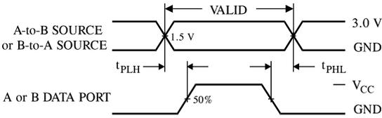
Figure 4. Switching Waveforms
