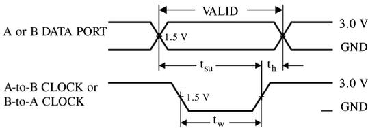
Figure 7. Switching Waveforms
