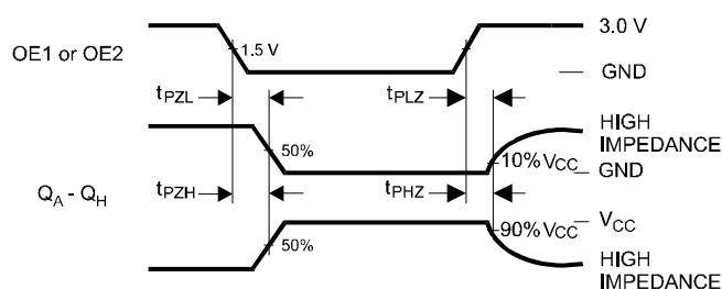
**Figure 3. Switching Waveform**
