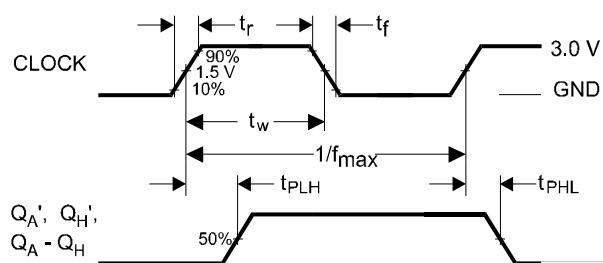
**Figure 1. Switching Waveform**
