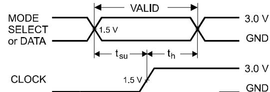
**Figure 4. Switching Waveform**
