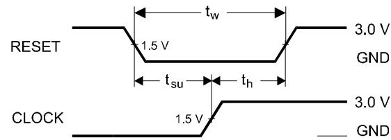
**Figure 2. Switching Waveform**
