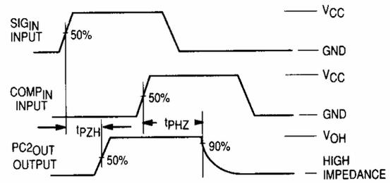
Figure 2. Switching Waveforms
