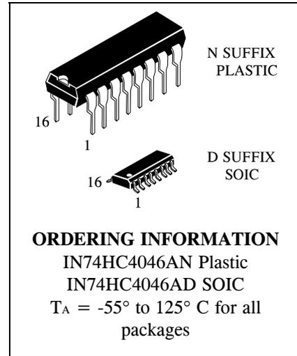
Applications include FM and FSK modulation and demodulation, frequency synthesis and multiplication, frequency discrimination, tone decoding, data synchronization and conditioning, voltage-to-frequency conversion and motor speed control.
