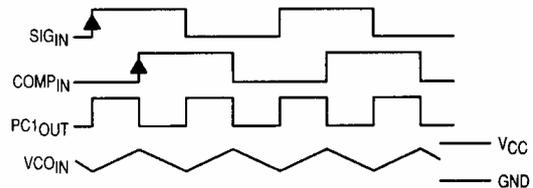
**Figure 7. Typical Waveforms for PLL Using Phase Comparator 1**
