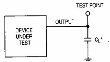
\*INCLUDES ALL PROBE AND JIG CAPACITANCE
