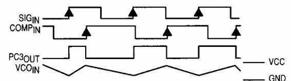
**Figure 9. Typical Waveforms for PLL Using Phase Comparator 3**
