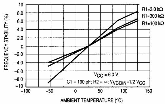
Figure 11C. Frequency Stability versus Ambient Temperature:  $V_{CC} = 6.0 V$
