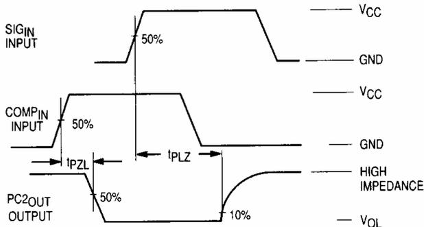
Figure 3. Switching Waveforms
