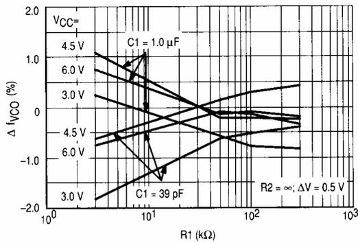
Figure 13A. Frequency Linearity versus  $R_1, C_1$  and  $V_{CC}$
