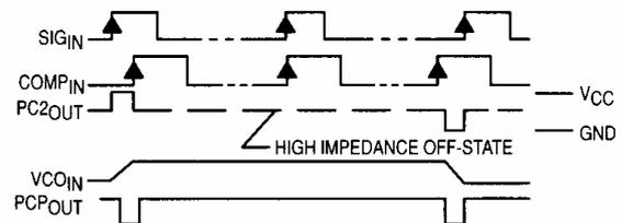
**Figure 8. Typical Waveforms for PLL Using Phase Comparator 2**
