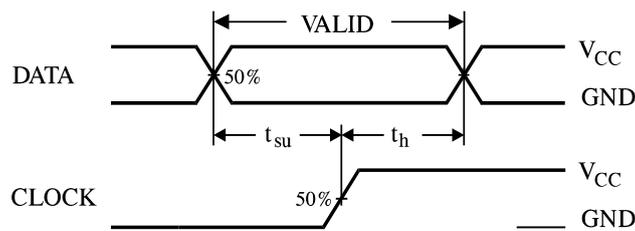
Figure 3. Switching Waveform
