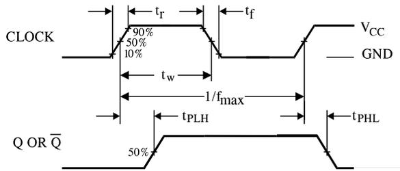
Figure 1. Switching Waveform
