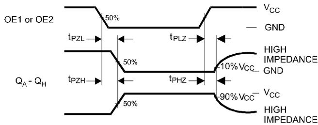
Figure 3. Switching Waveform
