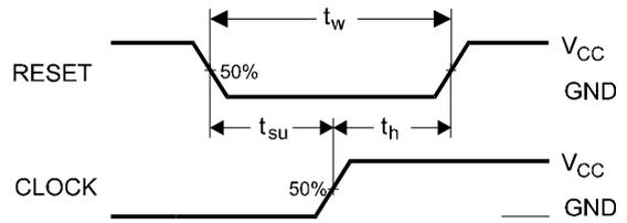
Figure 2. Switching Waveform
